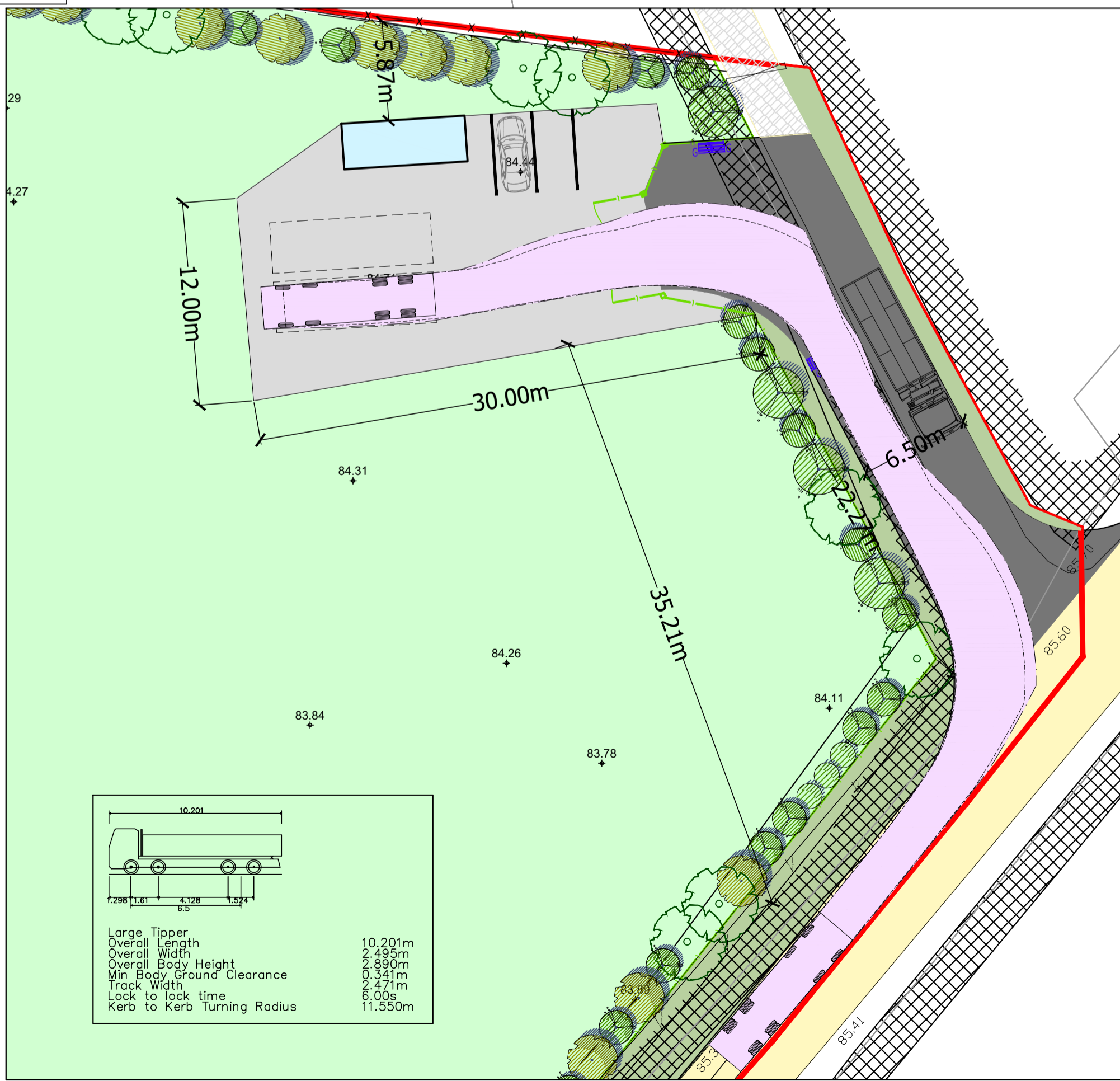
PROPOSED SWEEP PATH LARGE TIPPER (10.2m LENGTH) SCALE 1:250
